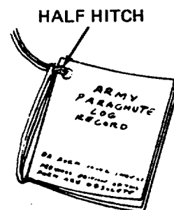
D. LOG RECORD ATTACHMENT TIE COMPLETED.
